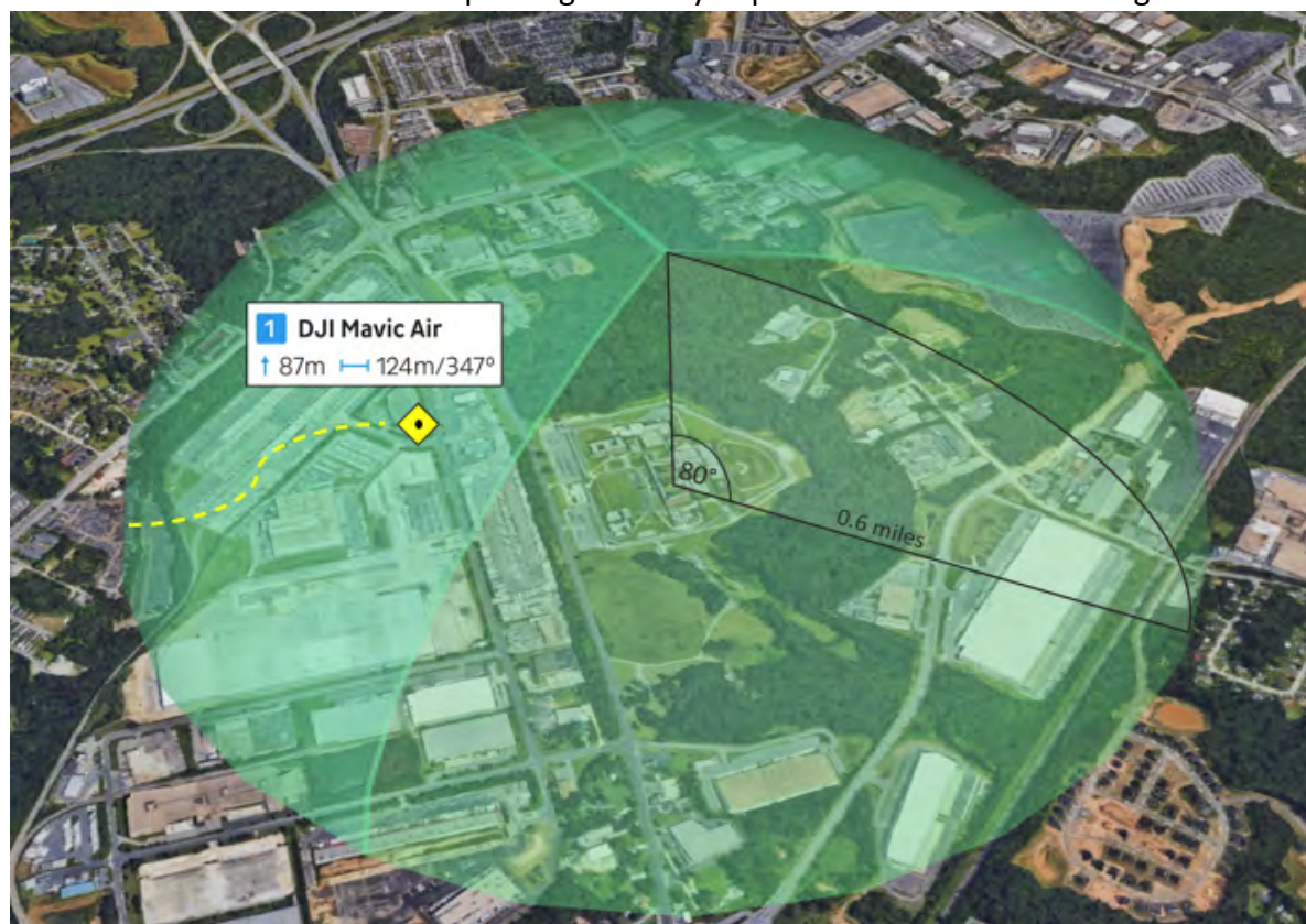
Figure 9. Depiction of DroneTracker 3D Radar Coverage. Radar provides the added benefit of detecting non-conventional drones (e.g. non-commercial and open sources UAVs) and determining elevation should you require significantly improved PTZ camera tracking.
