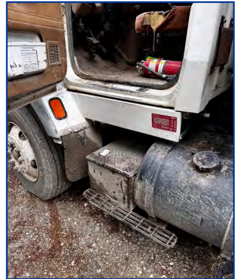
When exiting the water tender, the operator slipped on the diamond-plate step, falling approximately 4 to 4.5 feet. The fall caused an impact to the ribcage on the corner of the diamond plate step.
